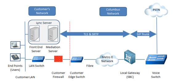
As shown in the diagram, SIP signalling traffic is transported from the Session Border Controller across the Columbus and Customer networks to the Mediation Server. If the trunk is encrypted Transport Layer Security (TLS) is used.
