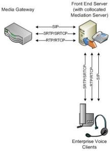
Lync Server 2013 supports greater flexibility in the definition of a trunk for call routing purposes from previous releases. A trunk is a logical association between a Mediation Server and listening port number with a gateway and a listening port number. This implies several things: A Mediation Server can have multiple trunks to the same gateway; a Mediation Server can have multiple trunks to different gateways; conversely a gateway can have multiple trunks to different Mediation Servers.
